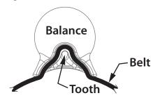
2. The belt is fully inserted when it slides behind the tooth and becomes captured in the slot.
