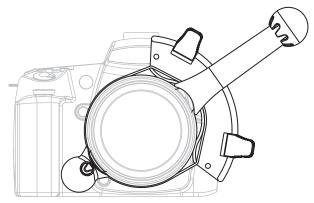
4. To remove the Balance, pull the belt out of the slot by wiggling it over the retaining tooth.
