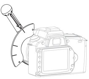
2. When using the hard stops, attach them onto the top edge of the marker board, at the focus stop positions. Position the marker board such that only the Focus Shifter arrow comes into contact with the hard stop.
